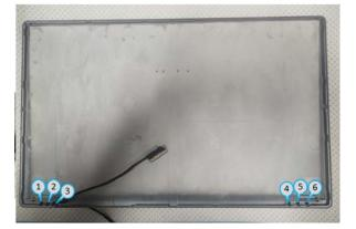
11.Take out the cablea: Tack out the cable from the back cover
